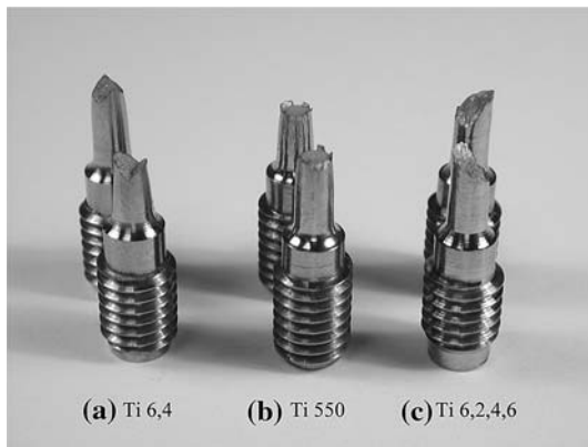
Fig. 4 Failed specimens after the quasi-static strain rate tests
